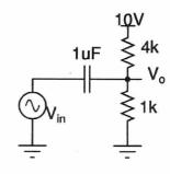
10. A) What is the voltage  $V_0$  when the frequency of  $V_{\rm in}$  is zero?
